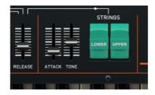
Above the "**release**" fader, you will find two other parameters available for the user. As the release, these parameters are applied on the Top Octave Divider oscillator, hence global for the Strings, Human voices or Vocoder carrier.
