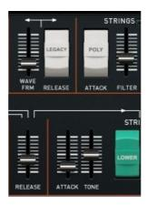
The rocker switch "**Legacy**", when on, allows the original hardware behaviour for the release: Each time the keyboard is empty; a new note will stop the current released sound.
