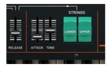
On the left of these two rocket switches, you will find two faders "**Attack**" and "**Tone**" which respectively set the Attack time of the strings and its high frequency characters.
