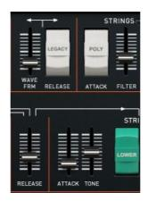
The rocker switch "**Legacy**", when on, allows the original hardware behaviour for the release: Each time the keyboard is empty; a new note will stop the current released sound.
