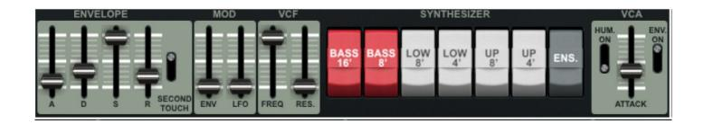
The **XILS 505** provides a full synthesizer section including a 24db self-oscillating ladder filter which can me modulated by an ADSR envelope and or a LFO through two independent amount set by the **ENV** and **LFO** faders.
