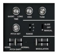
The "Pitch Shift" slider modulates when the three positions selector is set to "**Manual**" the pitch of the Top Octave Divider oscillator. This has the same behaviour as a standard pitch bend. The "**Pitch Set**" knob adjusts the amount of the pitch modulation.
