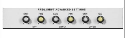
The frequency shifter is separated in two parts, each one as well as the dry path, has its one level and panoramic knob.
