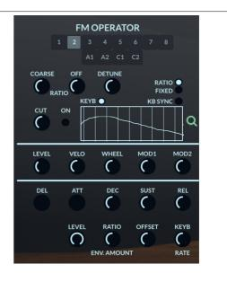
**RATIO:** This knob sets the ration used to calculate the operator frequency. For instance, a 2:1 ratio, and for a C3 note and when the current FM bank pitch is set to 0, then the operator frequency would be 261.62\*2 Hz = 523.24 Hz.
