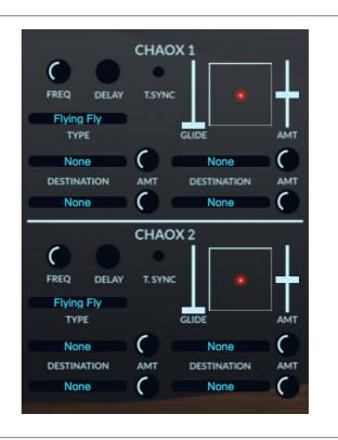
This exclusive module allows the addition of wonderful modulation like an LFO creates, but without the repetitive sound that standard cycle waveforms can give. The idea behind this module is to mimic reality. It's not exactly random, but without a repetitive cycle, just chaos!
