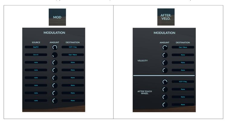
The source of the modulation can be the standard modulators, LFOs, Envelopes, Pressures, Velocity, and also one of the oscillators (Analog, Chaotic, FM) or the 4 track sequencer which can be used as a step modulator (see the list below).
