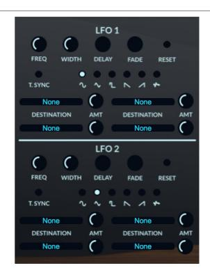
FREQ: Controls the speed of the modulation effect.
