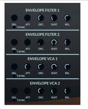
**DEL.**: Controls the time between the trig and the beginning of the Attack.
