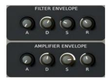
An envelope generator is a classic electronic module that outputs a command signal, built on four parts: ADSR (Attack-Decay-Sustain-Release).
