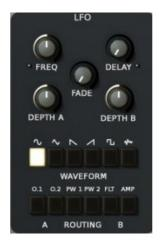
FREQ: Controls the speed of the modulation effect.
