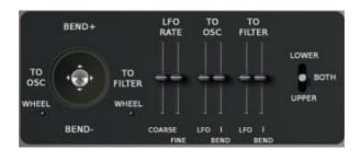
**LFO sliders :** Specify the coarse and fine tune of the monophonic low frequency oscillator. (Speed)
